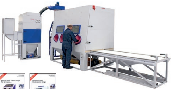
Euroblast 2.5 metre wide side loading cabinet side load facility for easier blasting of heavy or bulky components
